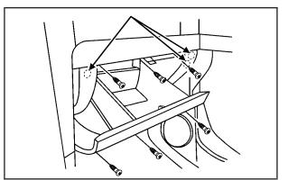
2. Lower the loosened glove box housing.
